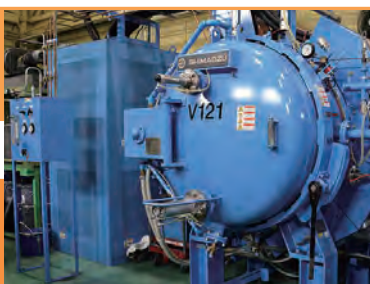
真空加压烧结炉 Vacuum pressurization sintering furnace
