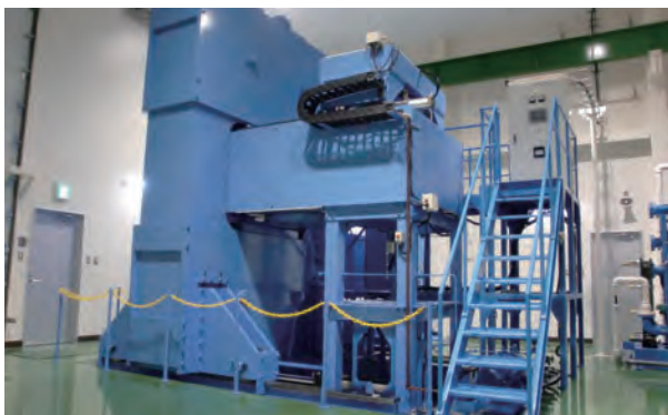
大型湿式CIP Large Wet Cold Isostatic Press
