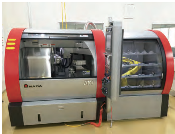
图形轮廓磨床 Graphical profile grinding machine
