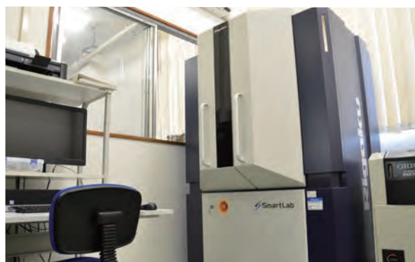
X射线衍射仪 X-ray diffractometer
