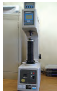
Rockwell 硬度计 Rockwell hardness tester
