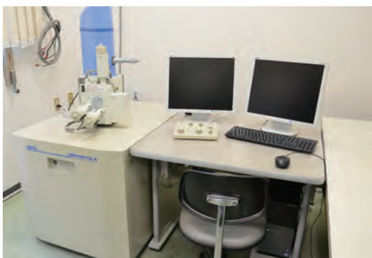
扫描电子显微镜 Scanning electron microscope
