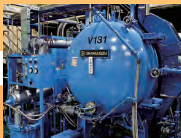
真空烧结炉 Vacuum sintering furnace
