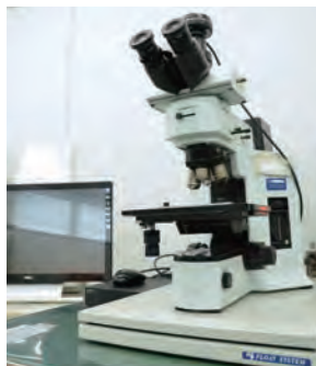
金属显微镜 Metallurgical microscope
