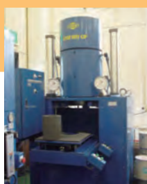
干式CIP Dry Cold Isostatic Pressing (CIP) device
