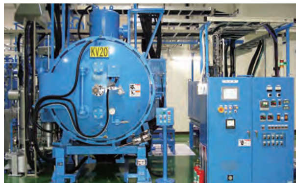
真空加压烧结炉 Vacuum pressurization dewaxing-sintering furnace
