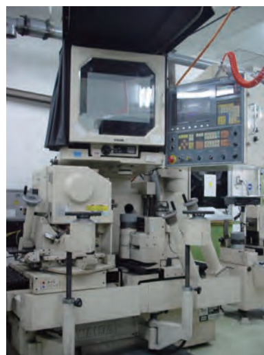
光学曲线磨床 Profile grinding machine
