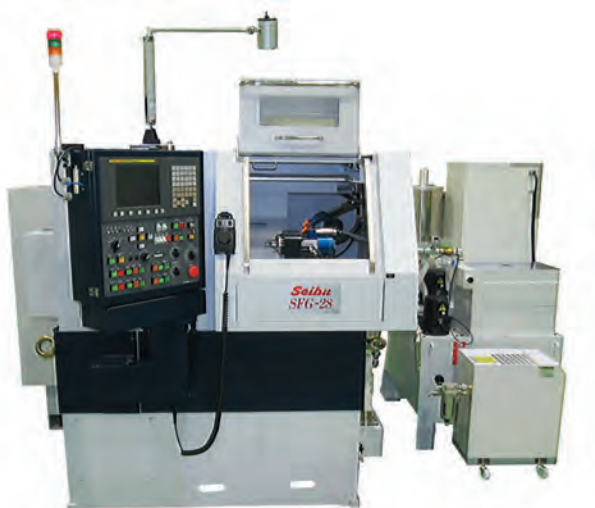
CNC精密内圆磨床 CNC internal cylindrical precision grinding machine
