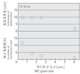
These figures show the relation between the WEDM process and the WC grain size of cemented carbide. It is revealed that the smaller the WC grain size becomes, the lower TRS after WEDM results. This is probably because the finer the alloy grains become the thicker the layer deteriorates after the WEDM process gets and more microscopic cracks are produced.
